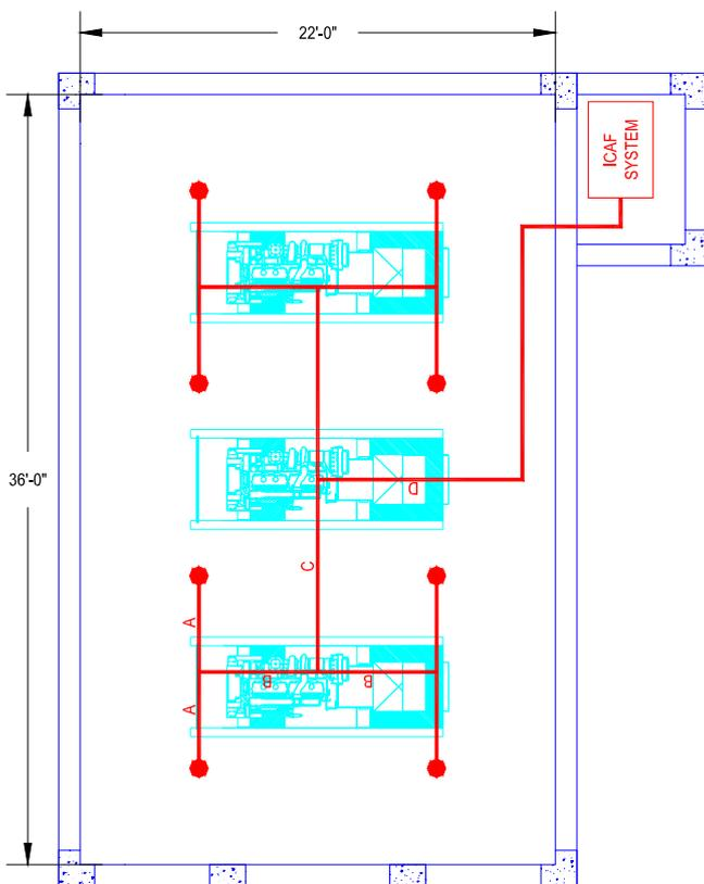
The ICAF system required for protecting this hazard includes a 10 gal. tank of foam concentrate with two (2) compressed air cylinders, representing a small footprint (see Fig. 2 below).
