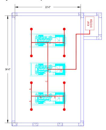
The ICAF system required for protecting this hazard includes a 10 gal. tank of foam concentrate with two (2) compressed air cylinders, representing a small foot print (see Fig. 2 below).
