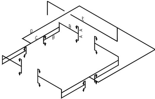
As shown above, the resulting balanced flow piping is much simpler to install and of smaller diameter than the equivalent deluge grid system, reducing the costs for the installing contractor.
